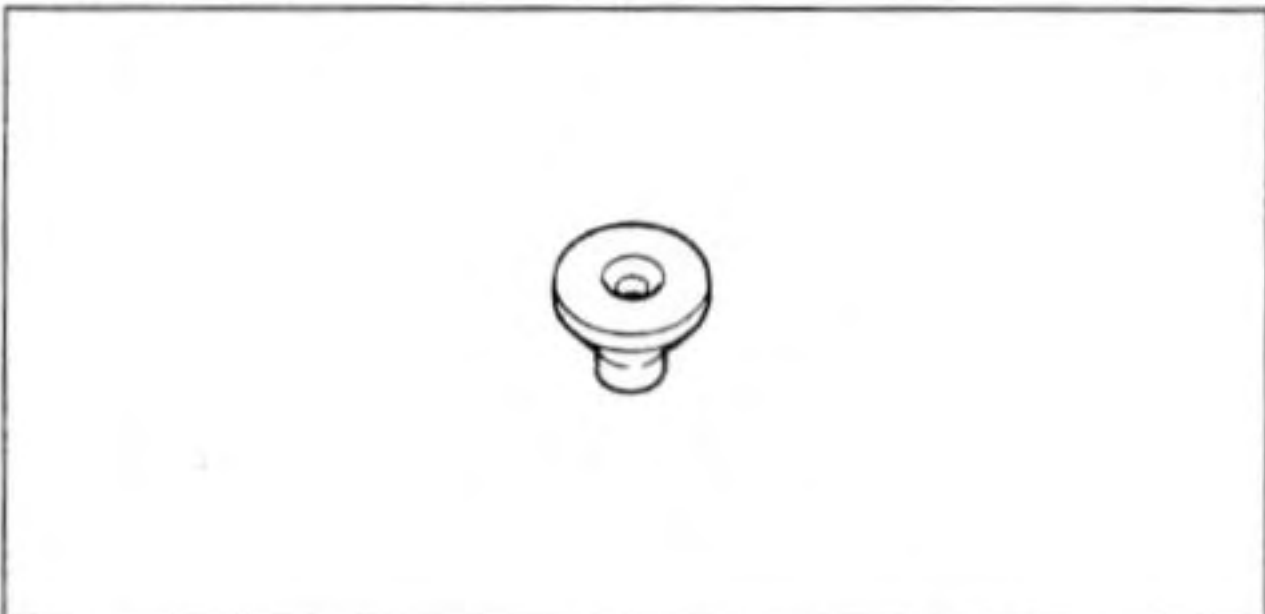
Head Pipe Outer Race Press Shaft: 57001-1075
